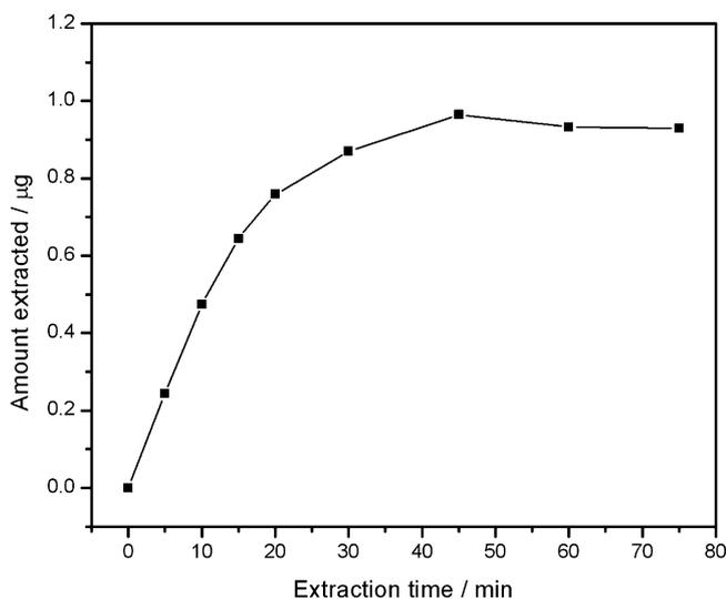
**Fig. 3.** Dependence of the extracted analyte amount on the extraction time. Sample: 0.57 μg/mL riboflavin in 10 mM sodium carbonate buffer, pH 10.0.
