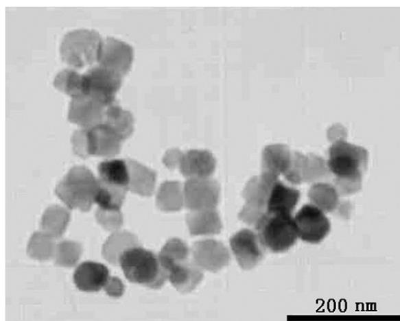
Fig. 1. TEM image of the boronate functionalized magnetic nanoparticles.
