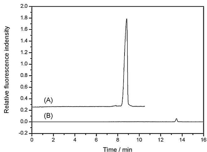
**Fig. 4.** Comparison of the peak of riboflavin in CE separation with (A) and without (B) pH junction. Sample: 5 μg/mL riboflavin in 20 mM phosphate buffer, pH 4.0; voltage, 15 kV; BGE, 20 mM sodium tetraborate, pH 10.0; gravity sample injection, (A) 30 cm for 120 s and (B) 10 cm for 10 s.
